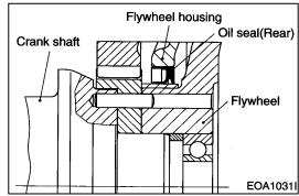
After fitting the flywheel housing holes to the guide pins and engage temporarily 2 ~ 3 threads of fixing bolts, and according to the tightening order (zigzag method) tighten them in the specified torque.
