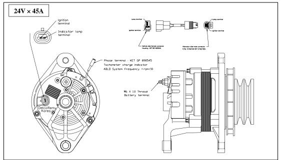
• The alternator is maintenance-free, nevertheless, it must be protected against dust and, above all, against moisture and water.
