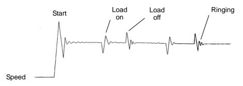
b) Optimum performance on load transients with slight overshoot on starts (optimum damping)
