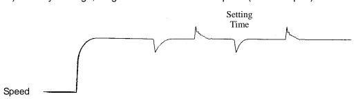
d) Stability too high, long time to settle to rated speed (over damped)
