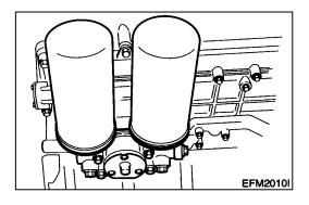
Lightly oil the O-ring and turn the oil filter until O-ring is fitted against the seal face.
