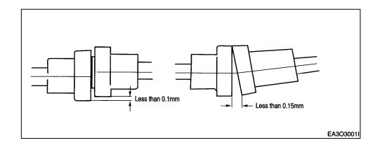
• For bed rail is apt to deform for 6 months after initial performance, adjusting the center should be checked after 1  $\sim$  2 months.
