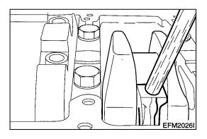
• By pushing the piston assembly with a wooden bar toward the cylinder head's direction remove the piston.
