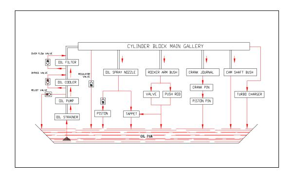
• Depending on the agreed extent of delivery and the design of the engine, the lube oil circuit can be equipped with oil pressure monitors (advance warning and cut-off function) which shut the engine down in the event of a sudden loss of pressure.
