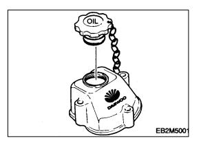
• For a few minutes, operate the engine at idling in order to circulate oil through lubrication system. Thereafter shut down the engine. After waiting for about 10 minutes measure the quantity of oil and refill the additional oil if necessary.
