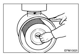
• A check should be made from time to time to see that the fastening elements securing the air cleaner to the intake manifold seal the connection tightly. Any ingress of unfiltered air is liable to cause a high rate of cylinder and piston wear.
