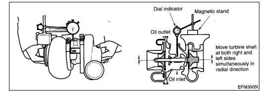
c) In case that the end plays to axial and circumference directions, replace or repair the turbocharger.
